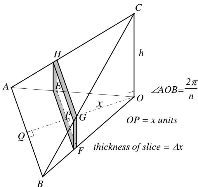
Consider a slice with cross-section  $EFGH$  perpendicular to the plane  $AOB$  with  $EF \parallel AB$ , thickness  $\Delta x$  and at a perpendicular distance  $x$  units along  $OQ$  from the point  $O$ .
